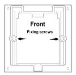
(c) Read the head panel and read the head body snap together, first from the upper snap down and then press the lower and bottom screw hole alignment; finally in the bottom of the anti-theft screw hole screwed on the countersunk head machine wire within the plum security screws fixed, as shown in the figure below.
