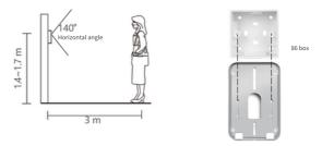
1. Drill holes for passing through the 4-core cable, it connects the outdoor phone and indoor monitor, interconnecting audio and video.
