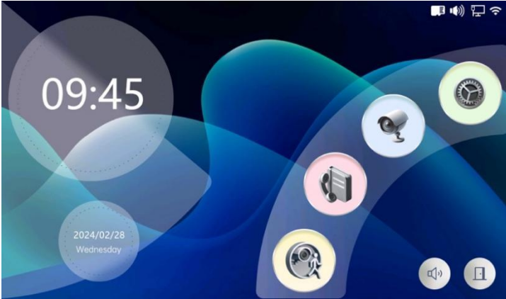
Image 2-1 indoor monitor operation main interface
