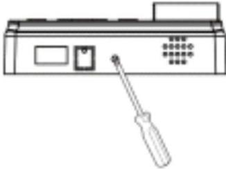
2. Remove the rear cover from the device.
