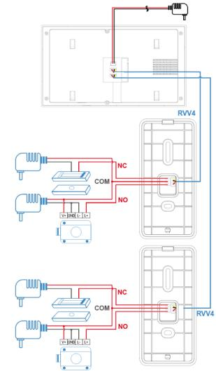
Figure 1-5 Standard Connection Diagram 2 Set Outdoor Station to 1 Set Indoor Monitor
