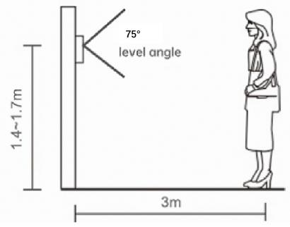
Figure 1-1 Outdoor Station Installation Diagram
