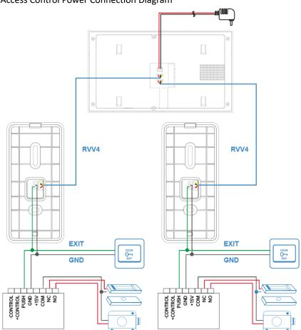
Access Control Power Connection Diagram
