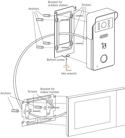
Figure 1-2 Device Installation Diagram
