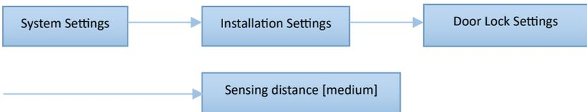
Note: Sensing distance [near]: about 30 to 50 cm; Sensing distance [medium]: 50 to 70 cm; Sensing distance [far]: 70 to 80 cm.
