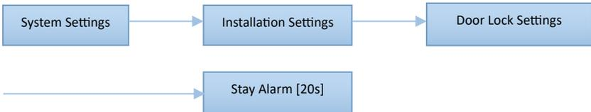
Note: If a person is detected for 20 seconds cumulatively within 1 minute, a stay alarm will be triggered. For the configured devices pushed, the sound and light alarm will not be activated by default.
