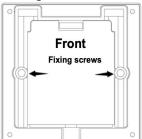
3 Read the head panel and read the head body snap together, first from the upper snap down and then press the lower and bottom screw hole alignment; finally in the bottom of the anti-theft screw hole screwed on the countersunk head machine wire within the plum security screws fixed, as shown in the figure below.
